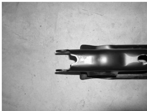
46. Install the factory torsion bar crossmember onto the Fabtech brackets. Note: on some trucks you will need to install the Fabtech torsion bar brackets and factory
