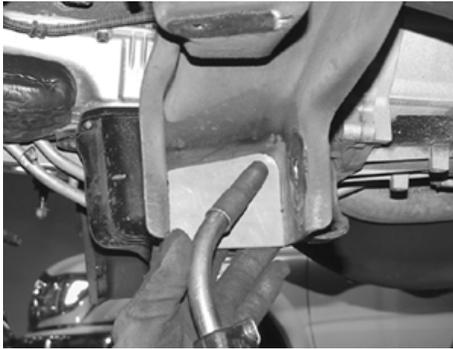
21. Locate and install the Fabtech rear crossmember into the factory lower control arm pockets using the stock hardware with the nuts towards the rear of the truck. Leave loose
