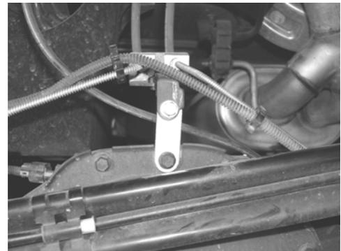
68. Raise the floor jack supporting the rear axle and slide the upper mount of the track bar into the drop bracket. Align the track bar with the lower hole and reinstall the factory bolt
