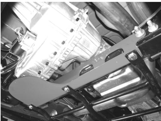
43. Recheck all bolts on the front end for proper torque before proceeding to next step.
