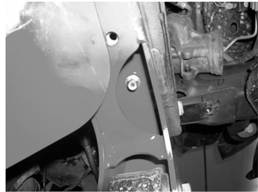
26. Position the front differential urethane bushing mount into the front crossmember tabs. Locate and install the differential skid plate around the differential housing bushing using the supplied 9/16"x 5" bolt, nut, and washers. Using the supplied 3/8" x 1" bolt and washer attach the rear of the skid plate to the rear crossmember. Leave loose. **If installing the optional Fabtech Full Differential Skid Plate FTS97000BK do so at this time, and discard the supplied FT20187 skid plate.**
