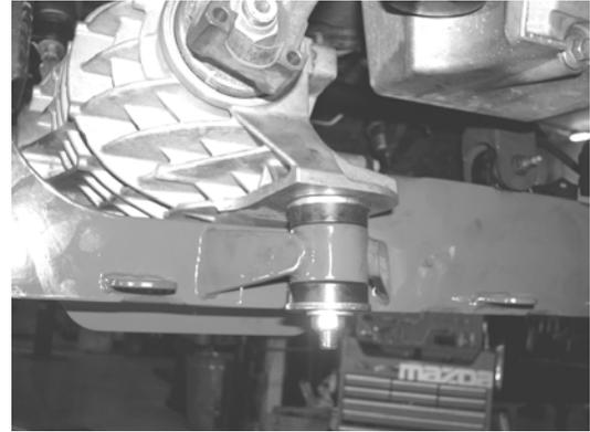
25. Locate and insert the square FT20058 tab bolts into the stock front control arm crossmember and through the holes outboard of the removed stock splash shield mounting holes. Attach the Fabtech front crossmember into the lower control arm pockets using the stock hardware. Use the 3/8" nuts and washers from hardware kit to attach the tab bolts to the under side of the crossmember. Leave loose. SEE PHOTO BELOW
