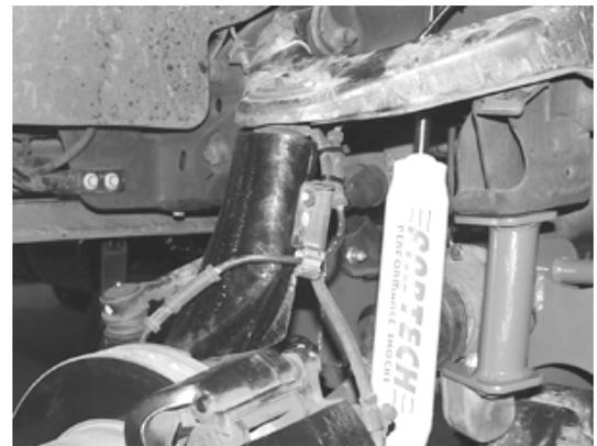
38. Install the new C.V. drive shaft FT20203 to the differential yoke using the stock hardware and torque u joint straps to 19 ft lbs.
