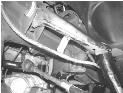
32. Locate the FTS20056D & P steering knuckle and install the stock hub bearing assembly taking care to place O ring in the proper position. Apply thread lock compound to the stock hardware torque the flange bolts to 130 lbs. SEE PHOTO BELOW.
