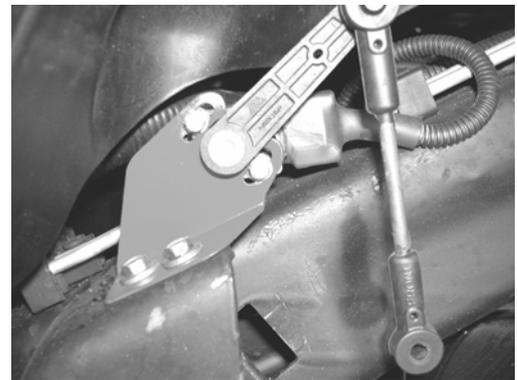
67. Install the brake line extension tab using the original bolt and the supplied 5/16" grade 5 hardware. SEE PHOTO BELOW.
