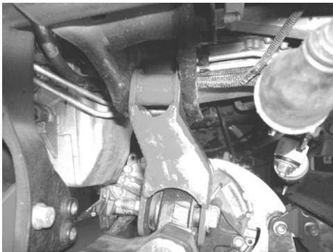
24. Place the differential housing into the Fabtech rear crossmember using the supplied 1/2" x 4 1/2" bolt, nut, and washers along with the supplied large FT55-1 washers attach the differential. SEE PHOTO NEXT COLUMN.
