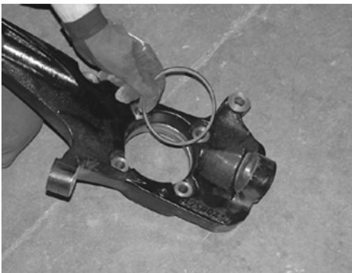
33. Working from the driver side of the truck, attach the steering knuckle FT20056D for the driver side to the upper control arm and to the lower control arm using the stock
