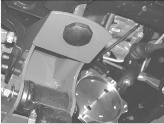
31. Locate the factory brake line mount on top of the upper control arm. Remove the brake line mount, and route the line with bracket to the bottom side of the control arm. Drill a guild hole directly below the original hole on the upper control arm. Mount the factory bracket to the bottom side of the control arm using the supplied 5/16 thread forming bolt. SEE PHOTO BELOW.
