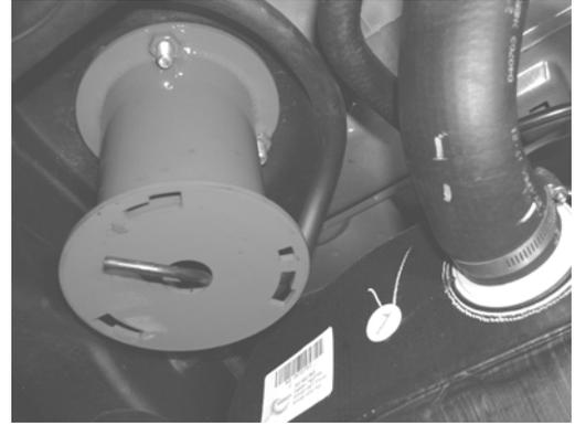
65. Reinstall the factory air bag onto the new spacer previously installed. The air bag will need to be locked into the spacer by engaging the tabs from the air bag to the spacer and twisting the air bag clockwise. Set the lower mount of the air bag onto the axle.
